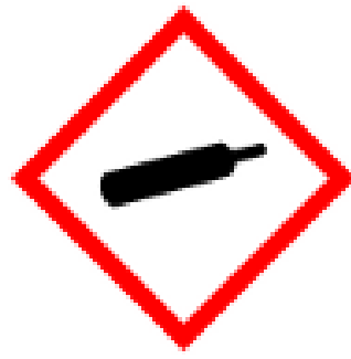
Gas Under Pressure
